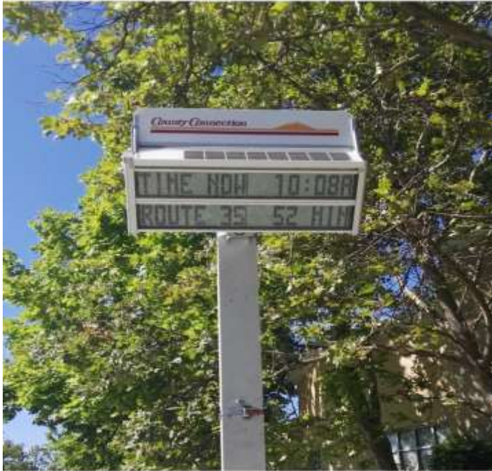
Figure 7. Wayside Solar Powered Next Bus Arrival Sign
